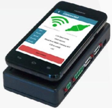
Nimbus Mobile is supplied in a portable carry case which includes a USB battery, auxiliary power cables and a USB power plug .
